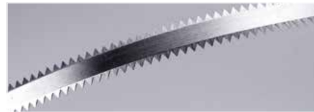
No 28 | 10 Teeth/inch; 10 x 0,45 mm | double pointed toothing
