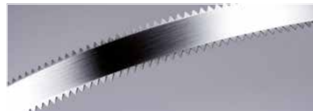
No 44 | 10 Teeth/inch; 15 x 0,45 mm C100S | double pointed toothing
