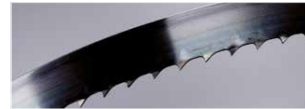
No 26 3 Teeth/inch; 20 x 0,80 mm angle tothing / set with broaching tooth
