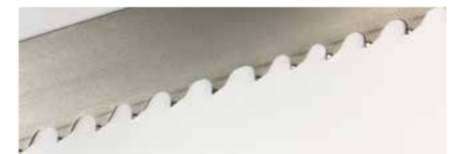
No 53 2/3 Teeth/inch; 27 x 0,90 mm angle tothing / not set, carbide tooth
