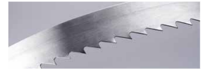
No 25 3 Teeth/inch; 20 x 0,50 mm angle tothing / set with broaching tooth
