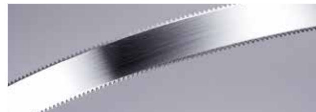
No 32 | 18 Teeth/inch; 15 x 0,45 mm | double pointed toothing
