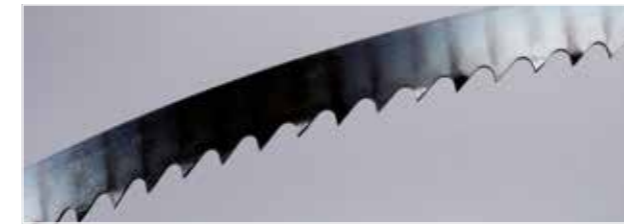
No 24 4 Teeth/inch; 13 x 0,65 mm angle tothing / set with broaching tooth
