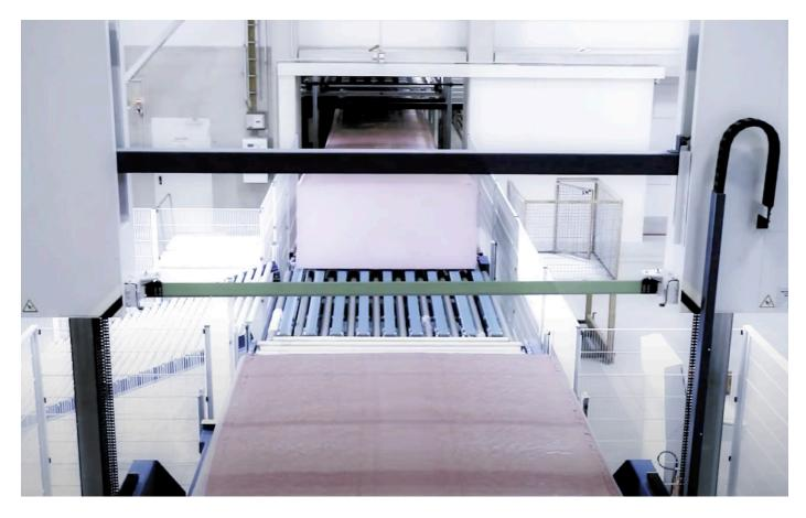
The continuously produced foam block is cut into long blocks. Usually, these blocks almost always have the same length of 30 meters. Tom would prefer that the blocks could be cut to length individually, depending on the orders. This would significantly improve the waste rate.
